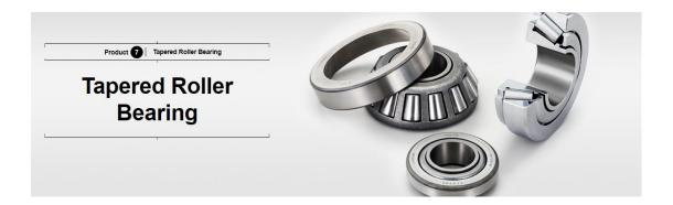
This bearing is designed so that the apex of the tapered face on the raceway face of the cone cup intersects with a single point on the bearing center line. Suitable for applications with heavy load and impact load.
